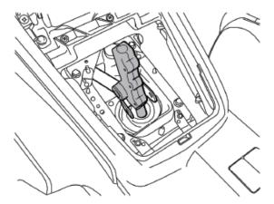
3. Before attaching to the shift linkage, apply a small amount of grease to both sides of the bushings used in the new shifter. There may be extra on the ball or socket to use.
