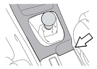
2. Use the two 12mm boxed end wrenches, one on either side, remove the bolt that holds the shift lever to the shift linkage as shown in the picture below. Do not misplace the nut and bolt, as they will be reused with the COBB Tuning Shift Lever.
