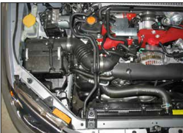
Factory air box system installed
