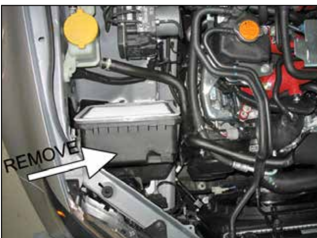
i. Remove the remaining half of the factory air box.
