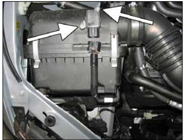
f. Remove the MAF sensor from the air box by removing the two screws. Set the MAF sensor aside in a safe area for later use.
