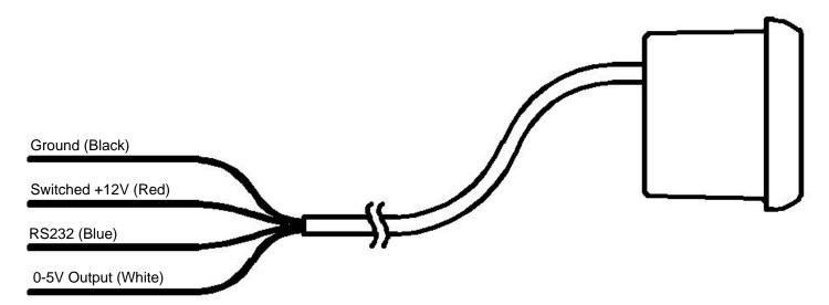
Figure 1. Connection Diagram
