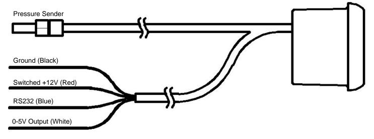
Figure 1. Connection Diagram
