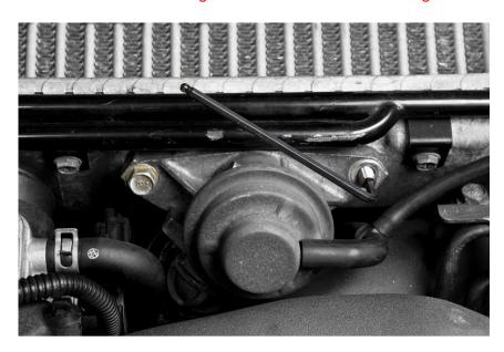
Step 3) Using the same 12mm wrench/socket, tighten the flange nut to 16 N-m (1.6 kgf-m, 11.7 ff-lb).
