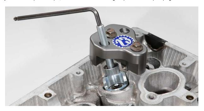
Step 5) Using the Company23 magnetic screwdriver's magnet, remove the valve spring keepers.
