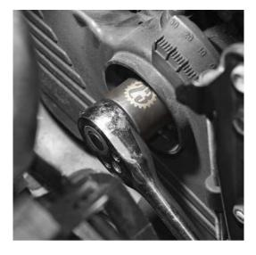
Step 3) Alw ays rotate the engine in a clockwise direction to prevent the timing belt from skipping.
