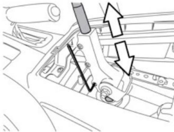
7. Remove the shift knob so that you can reinstall the center console shifter surround trim piece. Reinstall the center console shifter surround trim piece making sure to reattach the wiring harness for the lighter and screw the shift knob back into place making sure it is tight. Make sure the shift boot pops onto the lip of the shift knob.
