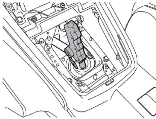
3. Before attaching to the shift linkage, apply a small amount of grease to both sides of the bushings used in the new shifter. There may be enough extra on the ball or socket to use.
