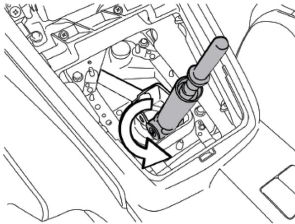
4. Remove the sleeve and bushings from the barrel of the factory lever. These will be reused with the COBB Tuning lever.
