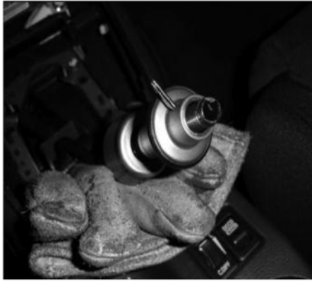
Driving the lockout pin out
