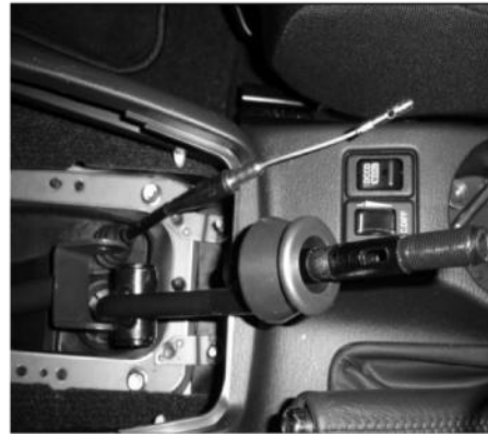
Cable removed from lever
