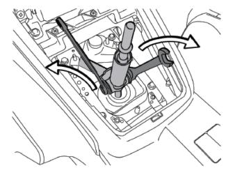
4. Next, remove the c-clip that holds the bottom cup in. You may have to purchase/borrow a pair of c-clip pliers in order to complete this step.
