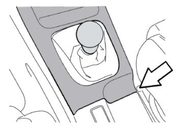
2. Disconnect the wiring harness for the lighter so that the surround can be placed aside. This will make it easier to work, without scratching the center console or the center console shifter surround trim piece.
