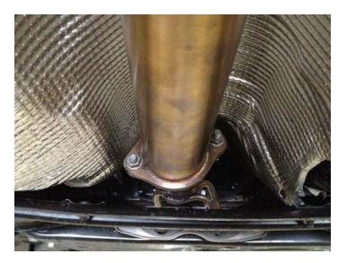
7. Now move on to the over-axle section of the exhaust. You'll need to snake the exhaust in from the back of the car. You'll likely need to bend/push the heat shielding to get the hangers through if you haven't already when removing the stock exhaust. Loosely install a gasket and 14mm hardware at the flange once you've installed it into the two rubber exhaust hangers.
