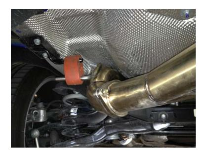
9. With the entire exhaust loosely installed, go back to the front of the exhaust and begin to tighten everything down. While exhausts seem to fit differently on every car, with three sections of this exhaust available to tweak/rotate, a perfect fit should be easily attainable. You're working to ensure the exhaust tips are level and centered in the outlet of the bumper. You may also play around with how the rods are fitted into the rubber hangers to get additional fitment options.
