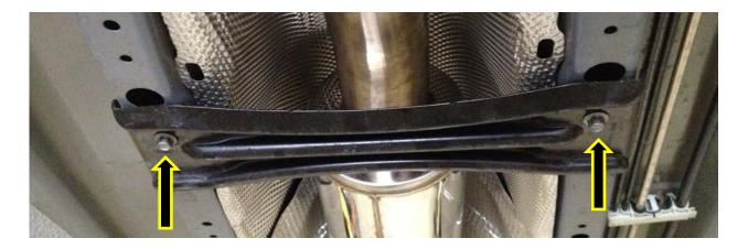
3. The Focus ST exhaust is a one-piece design. Because of this, you'll either need to drop the entire rear subframe and snake the exhaust out OR bring out the handy SawZall and get to work (which is what we suggest). You'll need to cut after the S-bend, right where the exhaust begins to rise to go over the rear subframe. See the picture below for reference. In this picture, we had already cut the exhaust off and welded in some v-band flanges for reinstallation for testing purposes.
