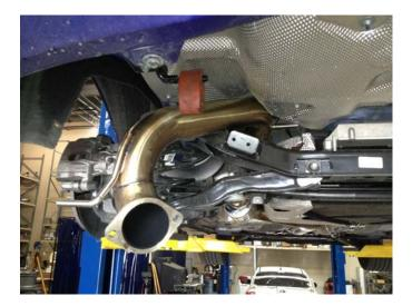
8. Now install the tip section onto the car by first installing the long rod into the rubber hanger on the passenger side of the vehicle. Once in place, loosely install a gasket and the supplied 14mm hardware to connect the two pieces.
