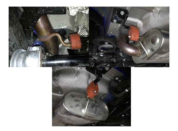
5. With the rear section removed, it's time to get the front section out. Using a 15mm socket and 15mm wrench, loosen and remove the two nuts that hold midpipe to the downpipe. Do not separate the flanges yet, though. There is a single rubber hanger at the apex of the S-bend that needs to be separated from the exhaust. Upon doing so, lower the exhaust down and pull it away from the downpipe to remove it from the vehicle.
