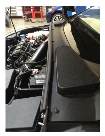
13. Underneath, there are two (2) 10mm fasteners holding the next layer of cowl in place. Remove them and remove the cowl.
