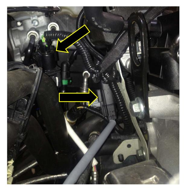
20. With the O2 sensor plugs removed, you can now remove the downpipe.
