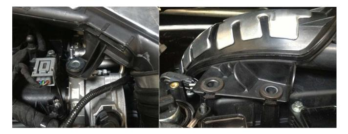
18. With everything loose, you should now be able to remove the intake tract. It may be easier to loosen the clamp in the middle of the tract and split it into two pieces to remove.
