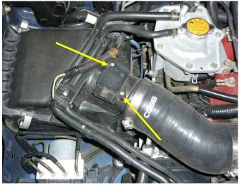
4. Remove the MAF sensor and set it aside.
