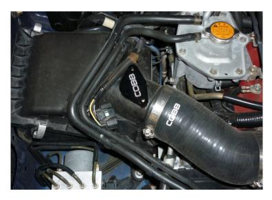
2. Using a M2.5 allen key, secure the Block Off Plate with the two M4 nylon washers and M4 button head cap screws. Hand tighten.
