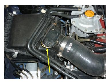
3. Using a M3 allen key (COBB SF Intake) or phillips head screwdriver (Stock Intake), remove the two screws that hold the MAF sensor to the MAF Housing.
