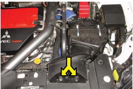
2. With the fasteners removed you may now remove the intake duct by pulling it straight out of the front of the air box.
