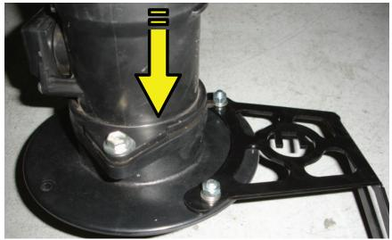
3. At this point you may now also attach the the COBB intake bracket to the MAF adapter using the supplied 10mm bolts, nut, and washers as shown.
