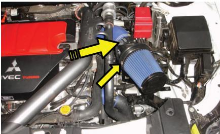
6. You have the option at this point to re install the factory inlet duct if desired using the two plastic phillips head fasteners.
