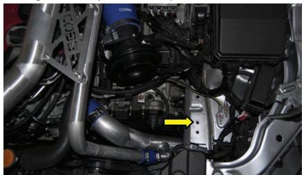
5. Now clip the MAF connector back into the MAF sensor choosing the best path for the wiring harness. Secure the filter on the end of the COBB MAF adapter using the supplied 8mm hose clamp and tighten, but do not over tighten the clamp as this may damage the clamp and/or the housing.
