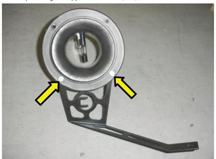
4. You may now install the MAF housing, adapter, bracket assembly in the car. Install the 13mm bolt and washer in the extra hole in the frame rail as shown and re-tighten the factory 10mm hose clamp.
