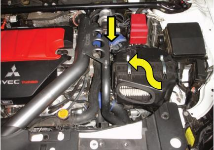
6. At this point using a small flat head screwdriver you will want to unclip the wire harness from the factory air box bracket as it will contact the COBB intake bracket. You also have the option at this point to remove the entire factory air box bracket (two 12mm bolts as shown) as it is not required with the COBB intake. You also can just leave it in place if you like. The stars show this optional step.
