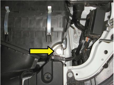
4. Now unclip the MAF sensor connector and the two plastic clips that secure the MAF sensor harness to the air box using a pair of needle nose pliers.
