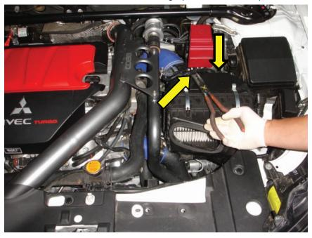
5. Now loosen the 10mm bolt on the hose clamp that secures the turbo inlet tube to the MAF sensor housing and you should be able to lift the factory air box and MAF sensor housing up and out.
