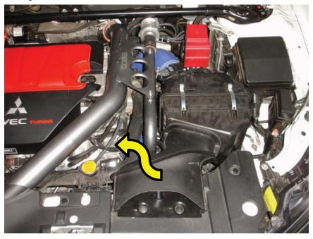
3. To remove the factory air box you will now need to remove the 10mm bolt located on the lower front side of the box.
