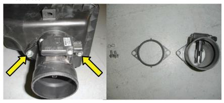
2. Attach the factory MAF housing to the COBB MAF adapter reusing the factory 10mm bolts. You may find it easier to install the rubber gasket into the COBB MAF adapter instead of placing it on the end of the MAF housing Don't forget to put the factory metal spacers inside the MAF housing when assembling. Tighten, but do not over tighten the 10mm bolts as this may cause the brass inserts to pull out of the MAF adapter.
