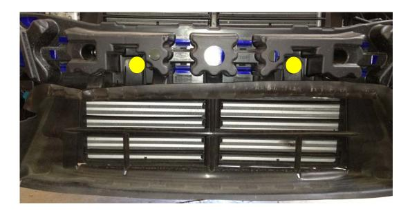
14. Disconnect the active grill shutter system on the driver's side. Plug shown below.
