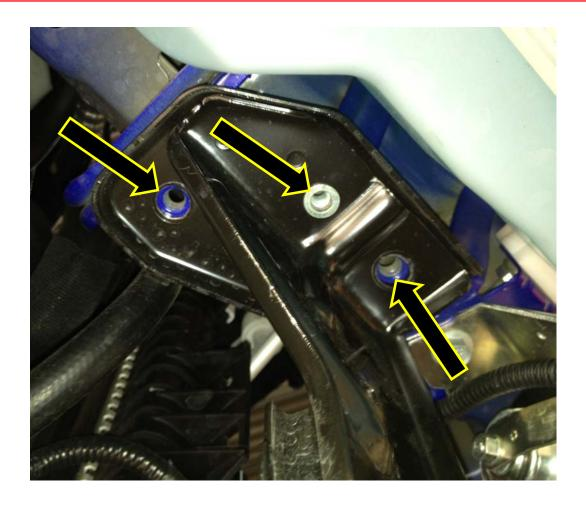
12. Using a 10mm socket, remove the two fasteners that hold the passenger side of the radiator support in place. You may also need to drill out a silver rivet to allow it to hang freely. (Some cars have this rivet and others haven't) Once loose, pull the rubber grommet out of the lower radiator support to allow the support to drop. This will allow you room to install the cold-side charge pipe connecting the passenger side of the core to the throttle body.
