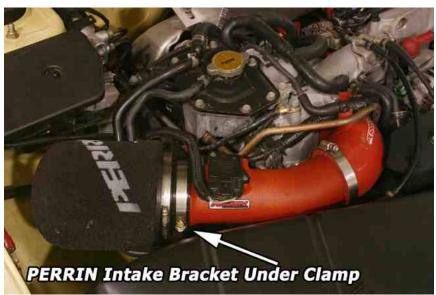
Above pic shows intake installed with optional PERRIN turbo inlet hose. NOTE: Supplied Silicone Coupler is not needed for this installation.
